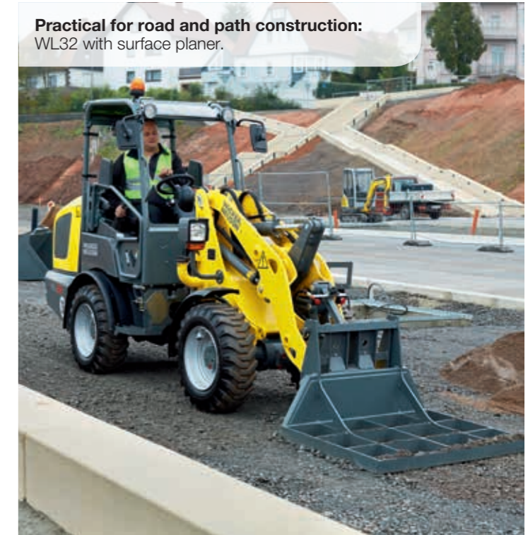
Two sturdy lift cylinders can take even large bucket volumes safely from A to B.
